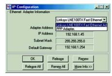
Figure B-1: IP Configuration Screen
