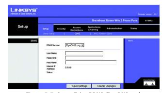
Figure 5-7: Setup Tab - DDNS (DynDNS.org)
