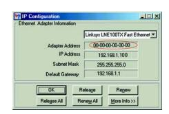
Figure B-2: MAC Address/Adapter Address
