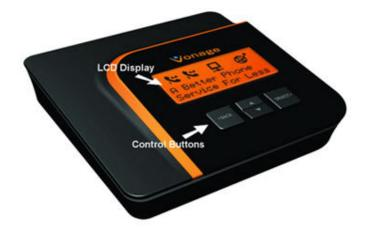
The V-Portal LCD display keeps you informed. From power-up through everyday use, the V-Portal communicates with you through the LCD display. <u>Status messages</u> are provided during power-up and use, letting you know exactly what is happening. The V-Portal even tells you when it is ready for you to use it for calling.
