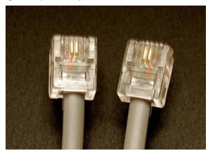
If you are using a two-line phone and you've activated both Vonage phone lines on your V-Portal, use a single standard four-wire telephone cord to connect your two-line phone to Phone Port 1 of
