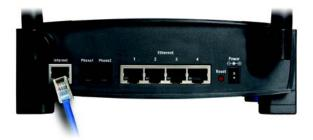
Figure 4-6: Connect the Broadband Modem
