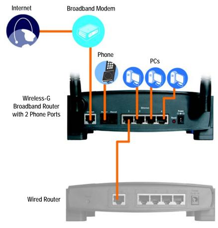
**Figure 4-5: Router Connected to Another Router**
