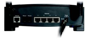
Figure 4-9: Connect the Power
