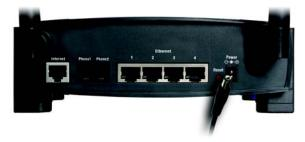
Figure 4-4: Connect the Power
