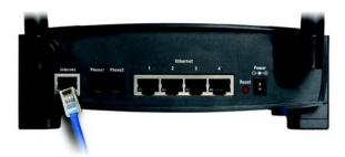
Figure 4-1: Connect the Broadband Modem
