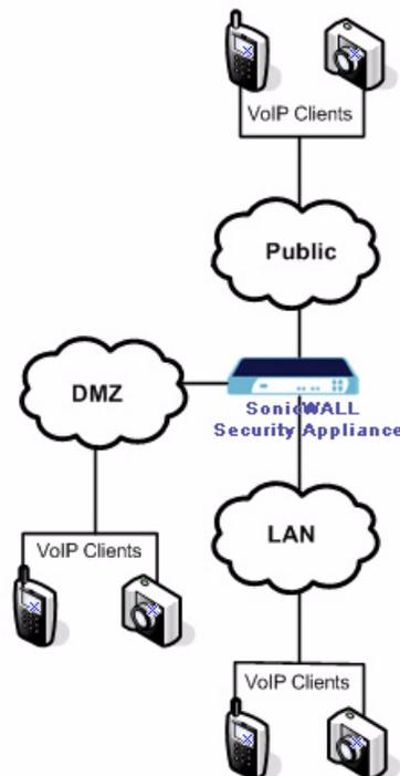
This deployment does not require a VoIP server. The Public IP address of the SonicWALL security appliance is used as the main VoIP number for hosts on the network. This requires a static Public IP address or the use of a Dynamic DNS service to make the public address available to callers from the WAN. Incoming call requests are routed through the SonicWALL security appliance using NAT, DHCP Server, and network access rules.
