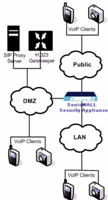
For VoIP clients that register with a server on the DMZ or LAN, the SonicWALL security appliance automatically manages NAT policies and access rules. The SonicWALL security appliance performs stateful monitoring of registration and permits incoming calls for clients while they remain registered. No configuration on the VoIP clients is required.
