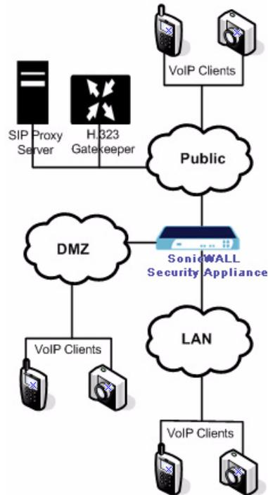
For VoIP clients that register with a server from the WAN, the SonicWALL security appliance automatically manages NAT policies and access rules. The SonicWALL security appliance performs stateful monitoring of registration and permits incoming calls for clients while they remain registered. No configuration of clients is required.
