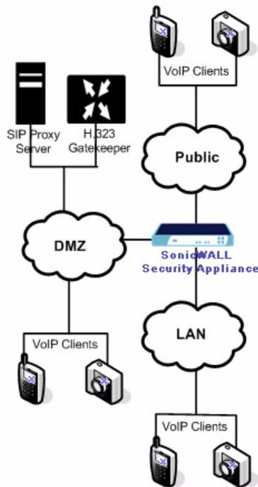
For VoIP clients that register with a server on the DMZ or LAN, the SonicWALL security appliance automatically manages NAT policies and access rules. The SonicWALL security appliance performs stateful monitoring of registration and permits incoming calls for clients while they remain registered. No configuration on the VoIP clients is required.
