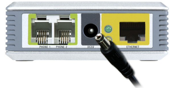
Figure 3-4: Connect the Power Adapter
