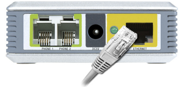
Figure 3-3: Connect the Ethernet Network Cable
