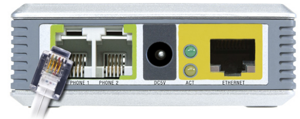
Figure 3-2: Connect the RJ-11 Telephone Cable
